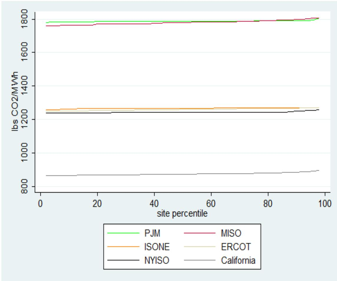
Notes: This figure displays the average marginal emissions displacement rates of individual sites over the entire study period within each region. Sites are arranged from lowest marginal emissions displacement on the left rate to highest on the right. See Section 5 for a description of marginal operation emissions approach.
