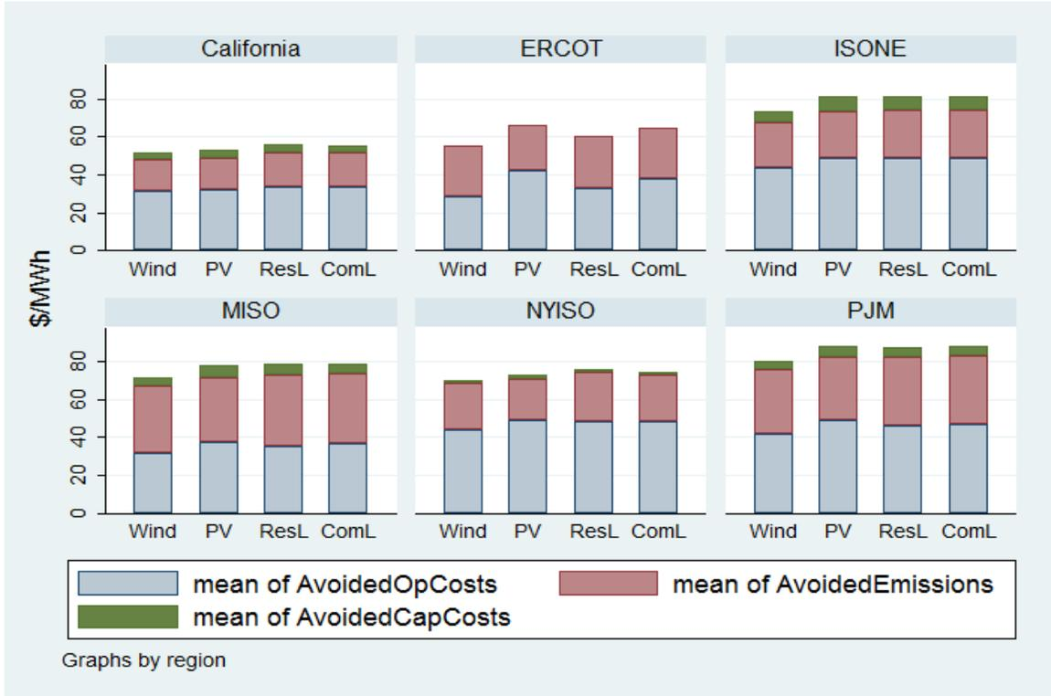
Notes: This figure summarizes point estimates of operating costs (in blue), emissions (in red; measured in monetary terms), and capacity value (in green) displaced per MWh of renewable energy generated or demand-side electricity saved.
