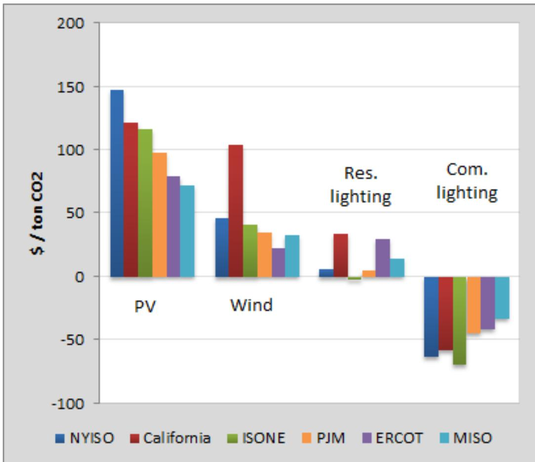
Notes: This figure plots the total marginal abatement cost, in dollars per ton of carbon dioxide, from different region-technology combinations under the assumption that only 50% of the estimated energy savings from lighting efficiency measures actually take place. See Section 7 for a description of marginal abatement cost calculations.
